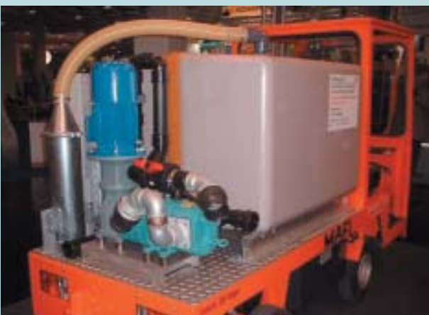
Boerger Rotary Lobe Pump on electrically driven mini truck with tank and filters. Mobile solution for the collection and discharge of sewage.
