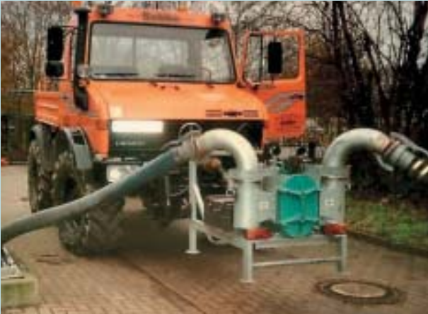
Truck with PTO drives a self priming Boerger Rotary Lobe Pump. High flows with small investment.
