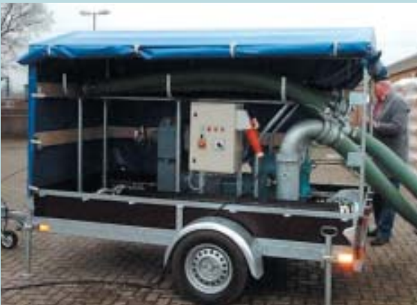
Boerger Rotary Lobe Pump with 350 gpm (80 m³/h) output on single axle trailer. Equipped with mechanically adjustable variable speed drive and rotatable flanges, compact and minimum weight.
