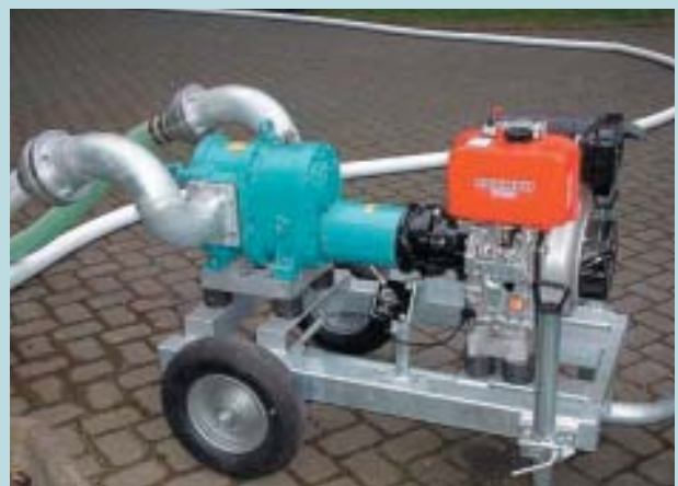
Mobile Boerger Rotary Lobe Pump on cart. Driven by single cylinder diesel engine.
