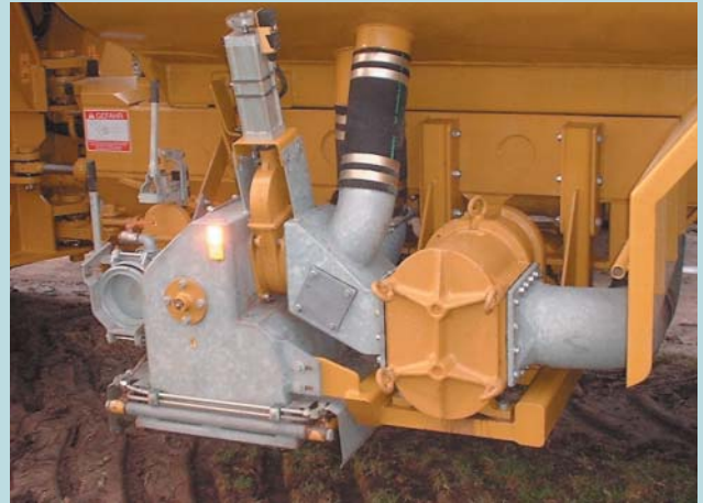
1,320 gpm (300 m 3 /h) truck mounted, hydraulically driven Boerger Rotary Lobe Pump. Minimum weight, high output, compact design and easy access. MIP = Maintenance In Place.
